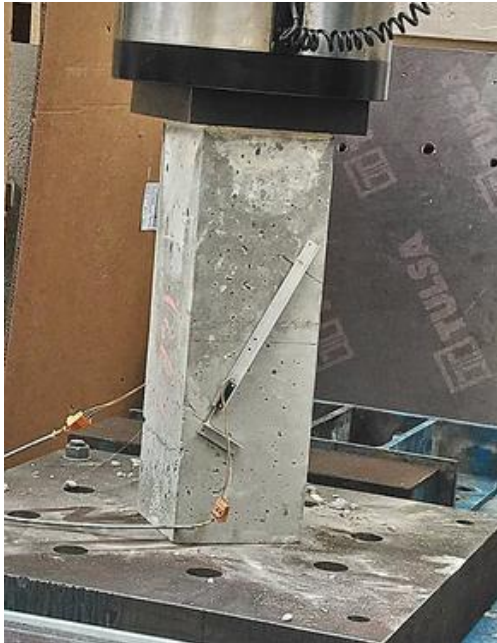
Figure 3.23 Slant shear test set up and instrumentation
