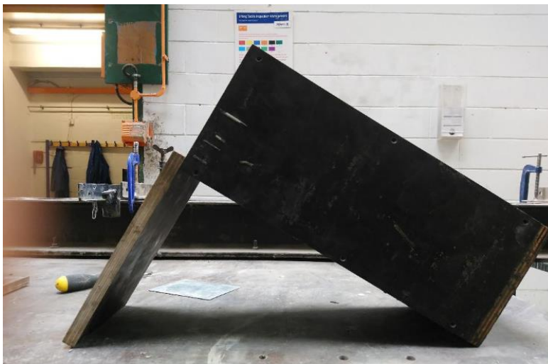
Figure 3.22 Wooden mould for placing the first layer of concrete
