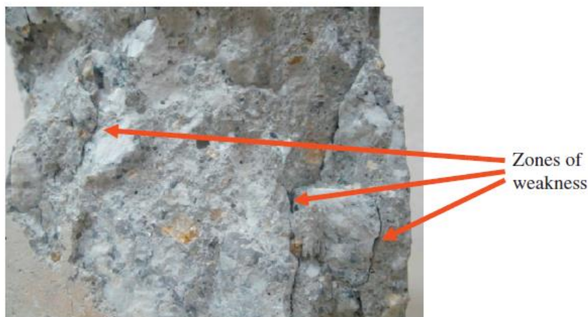
Figure 2.11 Crack pattern of recycled aggregates with attached cement matrix (Kwan et al., 2011).
