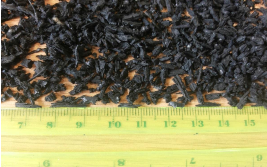
Figure 3.2 Crumb rubber (8mm length and 2mm thickness) particles from worn-out tyres
