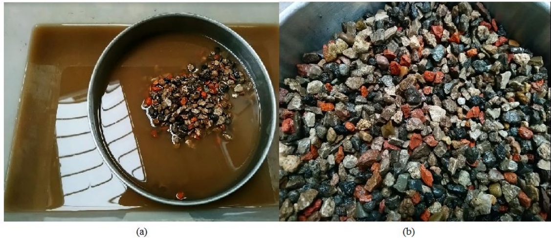
Figure 3.33(a) Washing set up of recycled aggregates (b) Washed recycled aggregates
