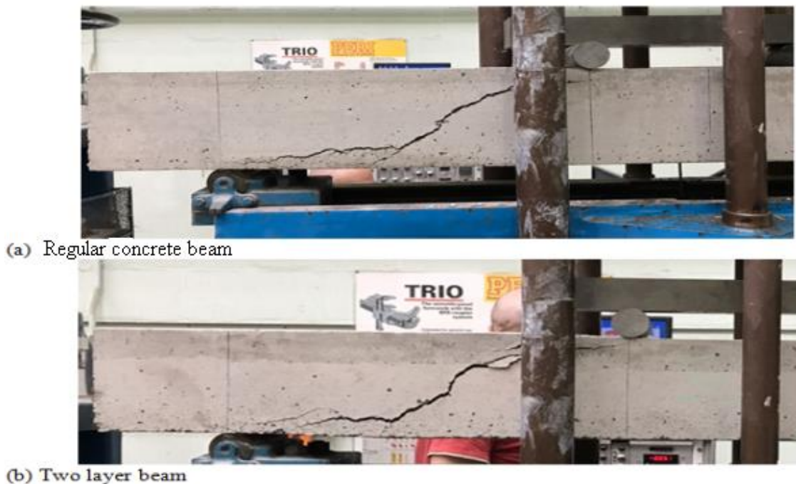
Figure 4.7 Failure modes of shear test beams
