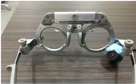
Figure 6.1 Video camera attached to the trial frame
