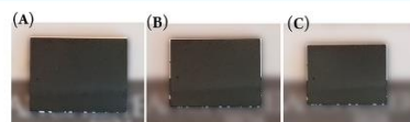
Figure 1. Photographs of an AACVD-grown (MAI+10%) MAPI film on ITO-glass substrate: (A) as-prepared, (B) after aging in ambient air for ~1 week, and (C) after aging in ambient air for ~1 month.
