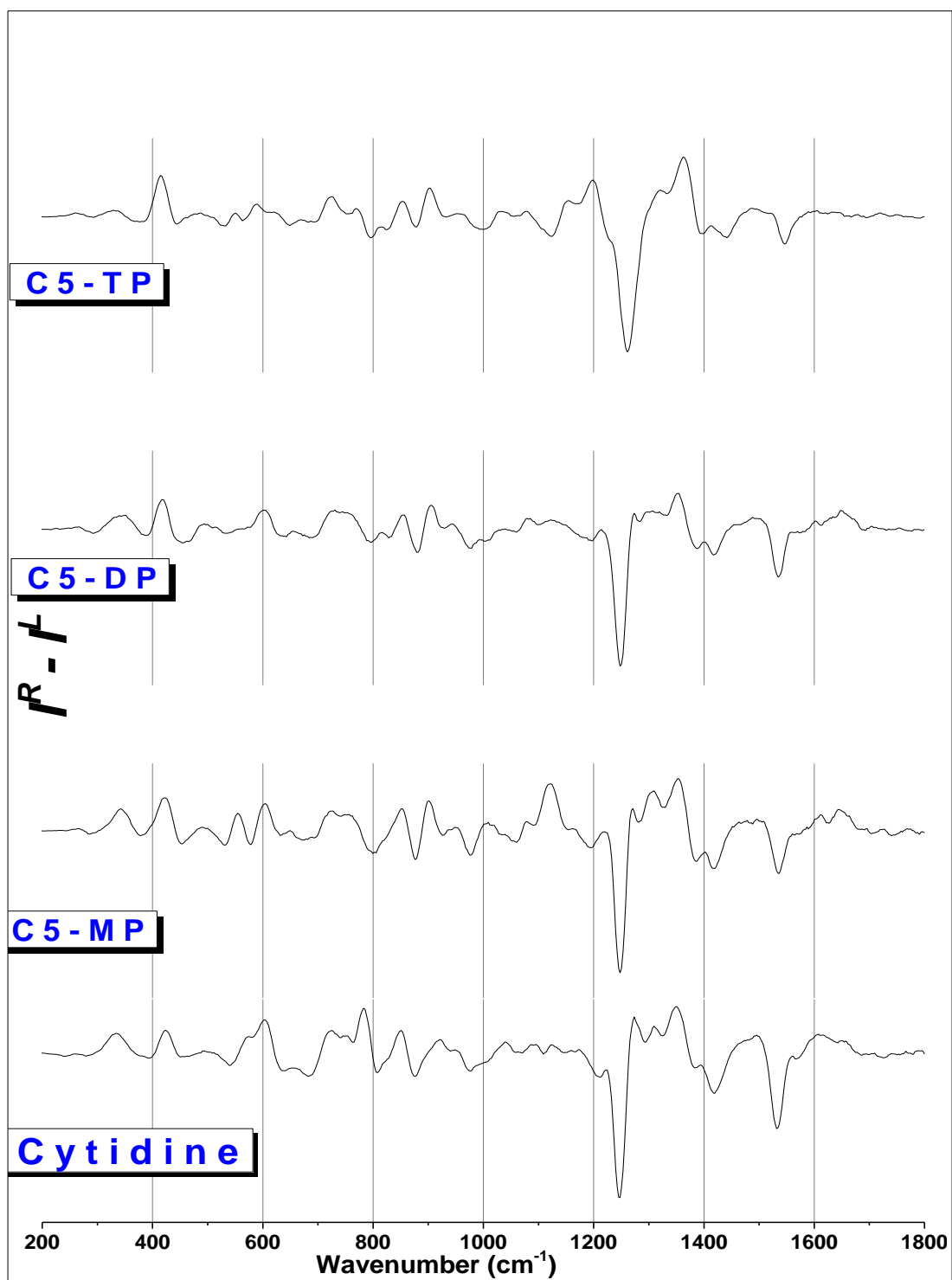
Figure 4.2. Raman optical activity ROA(I^R - I^L) spectra of Cytidine, Cytidine 5'-monophosphate (C5-MP), Cytidine 5'-diphosphate (C5-DP) and Cytidine 5'-triphosphate (C5-TP).
