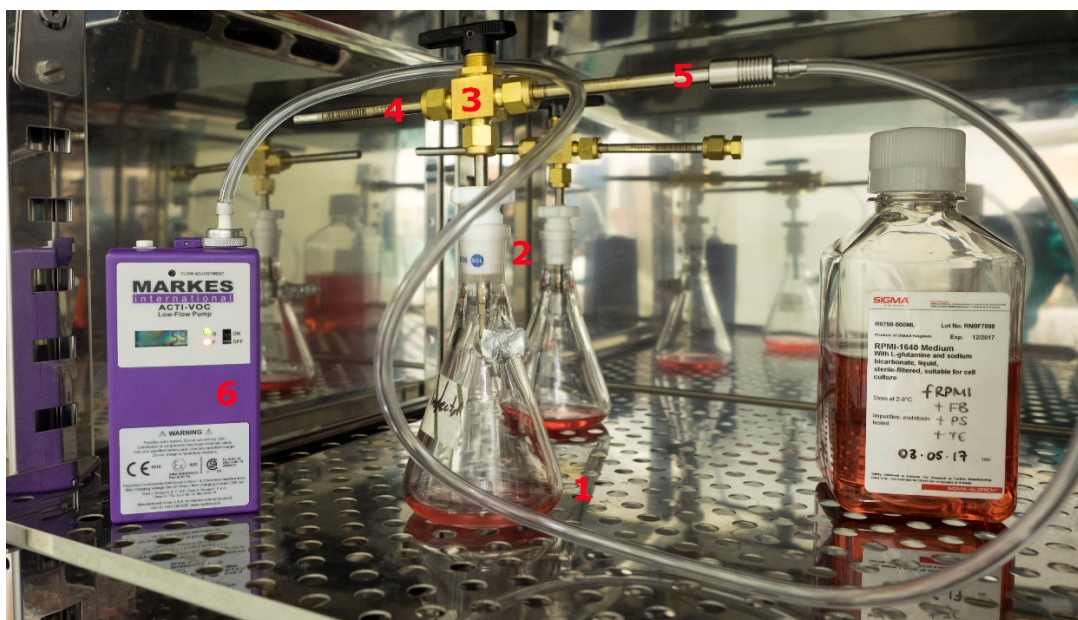
Figure 2.3 Experimental setup of the headspace sampling apparatus. A flask (1) containing the media with the fungal samples was sealed with a PTFE stopper (2) to prevent any gas leaks. The three-way stainless valve (3) was used to direct flow accordingly. A tube was placed to gather any VOCs passively up until the sampling time point (4) at which point the valve was switched to permit flow to the active sampling tube (5). Active sampling was achieved by vacuum suction by the Acti-VOC low-flow pump at 50 ml/min to avoid turbulence and VOC degradation.
