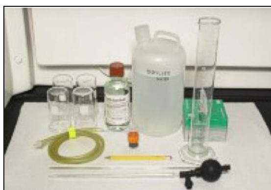
Figure 3.8: Photo shows materials required for carbonates removal with acetic acid. And these materials include: glacial acetic acid, distilled water, glass graduated cylinder, glass rod, 250-500 ml glass beakers, pipette, and siphon (Poppe et al., 2001).
