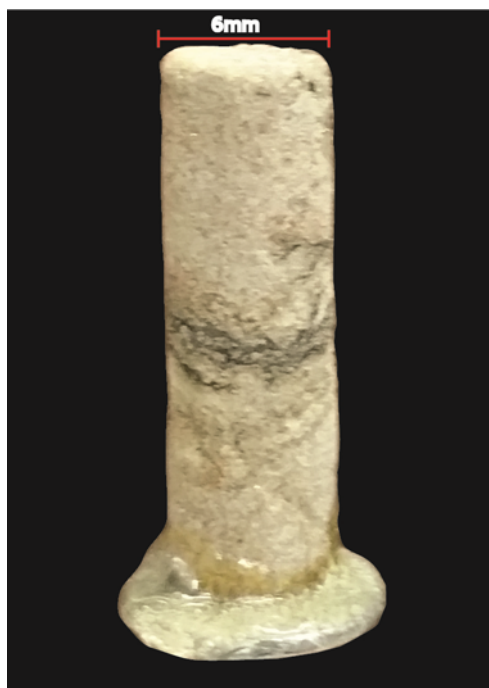
Figure 6.2: Core sample taken from larger sample. This sample was cut using rotary cutting tool. The core diameter is 6mm.
