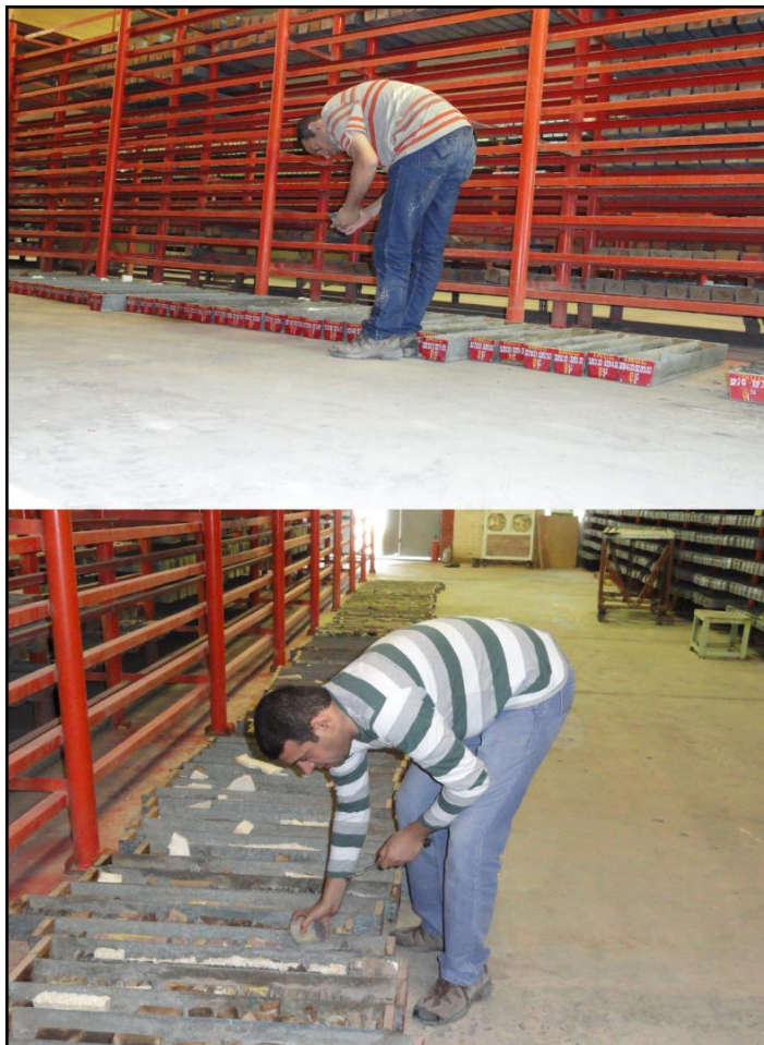
Figure 3.1: Systematic core descriptions in Core workshop at S.O.C, Iraq. Log-core depth calibration were applied to the cored intervals prior to start sampling and core visual core description
