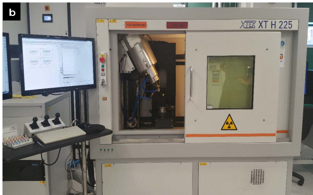
Figure 6.3: (b) Nikon Metris XTH 225 X-ray CT scanner, which was used to image core samples of the study area. The X-ray scanner is connected to the control workstation, which is used to adjust scan setting, data collection, data format and export to a storage hard drive.
