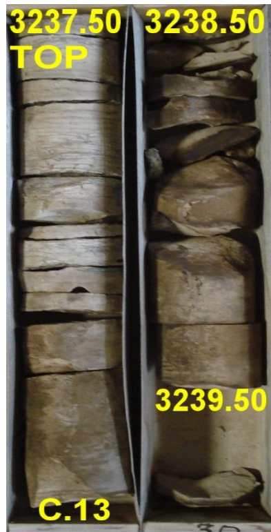
Representative core photos pf Well B North Rumaila Oilfield -Iraq
