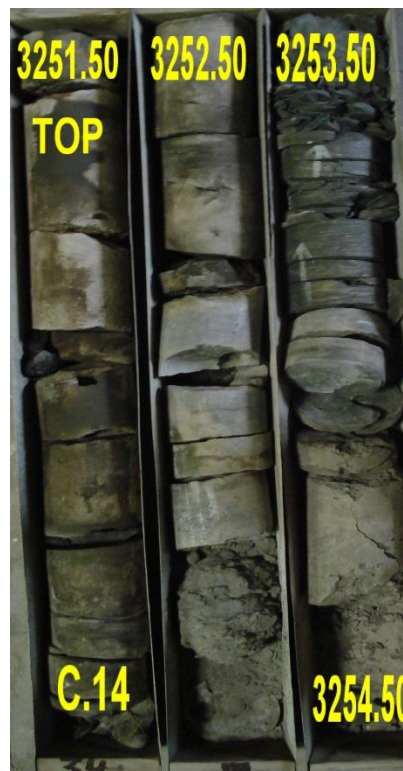
Representative core photos pf Well B North Rumaila Oilfield -Iraq
