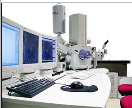
Figure 3.4: Environmental Scanning Electron Microscope FEI XL30 ESEM -FEG located in School of Earth and Environmental Sciences, The University of Manchester. This microscope is designed to work on Hi and Low VAC.
