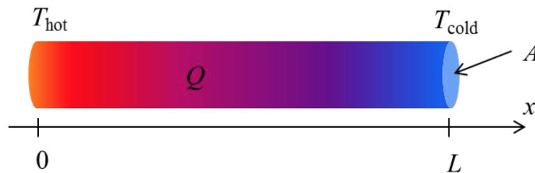
Figure 2.7: Conductive heat transfer in the one-dimensional case for a medium of constant cross-section A and length L [95]
