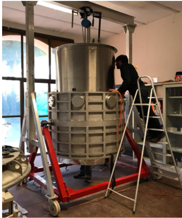
Figure 3.3: 40 K shield mounting in cryostat. Image courtesy: S. Masi.
