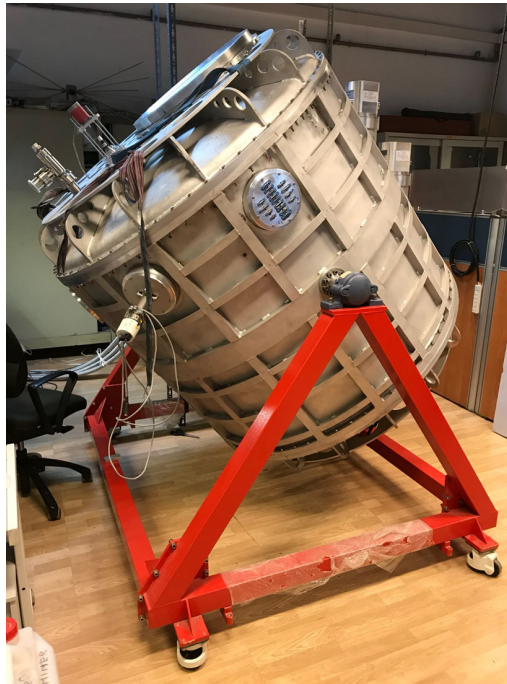
Figure 3.4: Closed cryostat under test. Image courtesy: S. Masi.
