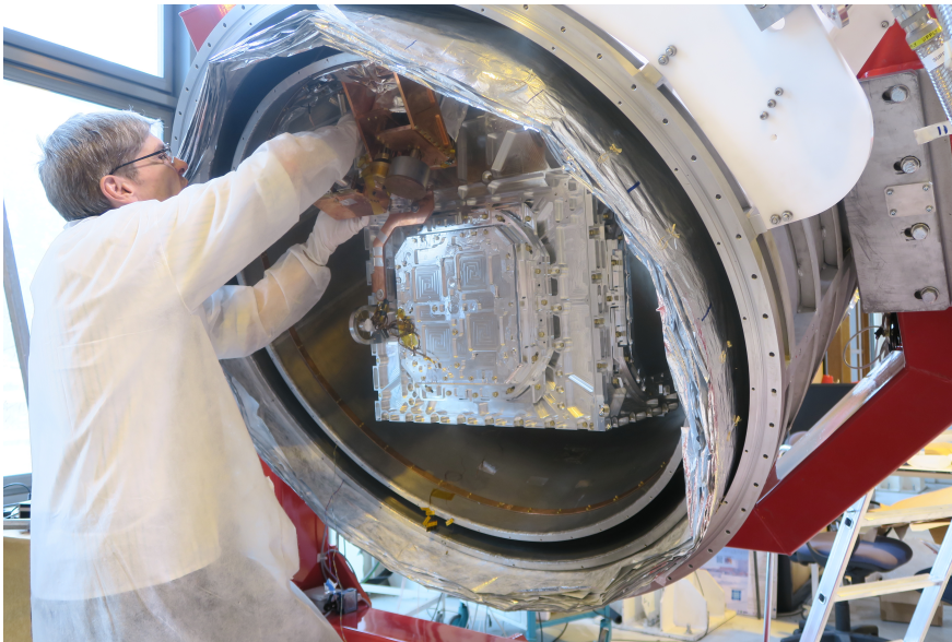
Figure 3.28: Installation of both sorption coolers with the 1 K box. Image courtesy: S. Torchinsky.
