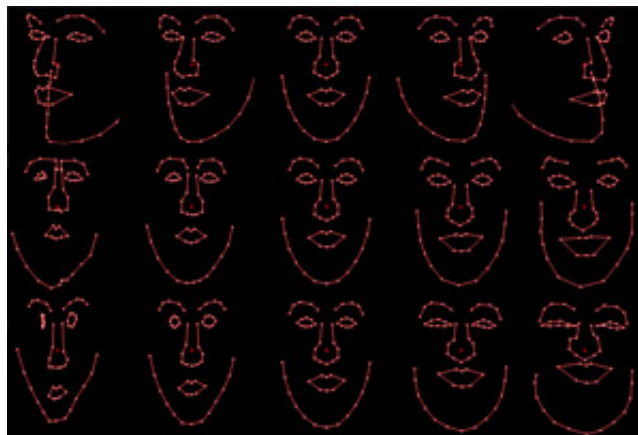
Figure 3.1: An example of three modes of a shape model.
