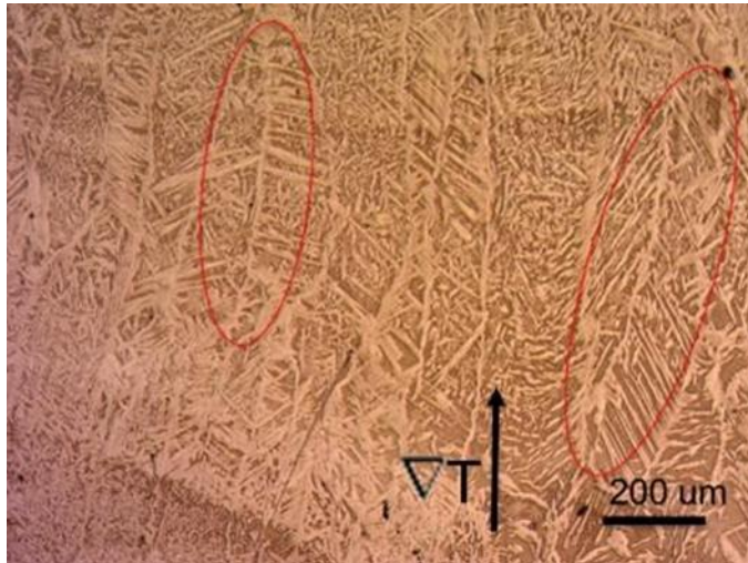
Figure 31 - Micrograph of the weld pass 1 after KOH etching.
