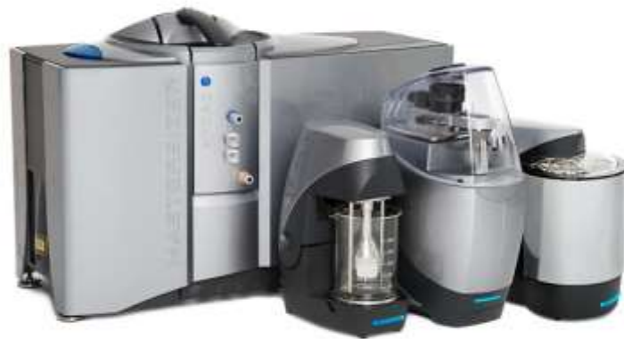
Figure 12: Malvern Mastersizer 3000 [49] used for analysing the particle size distribution of a given sludge sample. It is a laboratory based instrument which works on the principle of laser diffraction.
