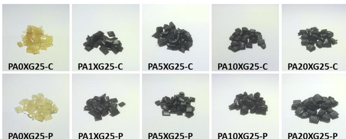
Figure 4.3. Photographs of melt processed PA11/GNP nanocomposites following extrusion and chopping, labelled appropriately.
