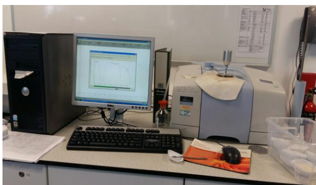
Figure 3.6: FTIR equipment for measuring change in absorbance of amide functional group hydrolysis in polymers [144]
