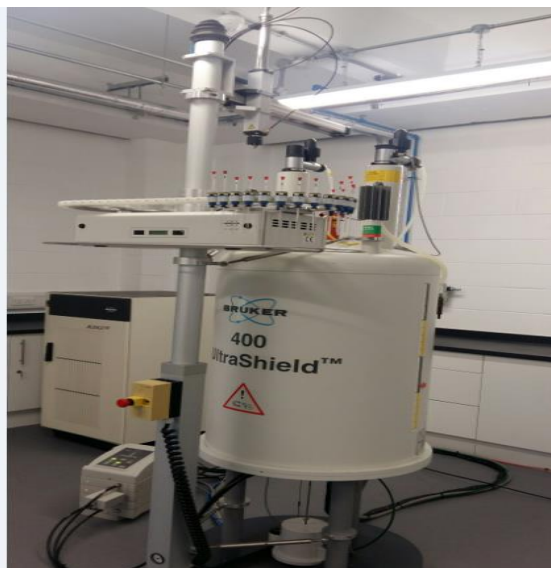
Figure 3.5a. NMR equipment for polymers degree of hydrolysis testing [144]
