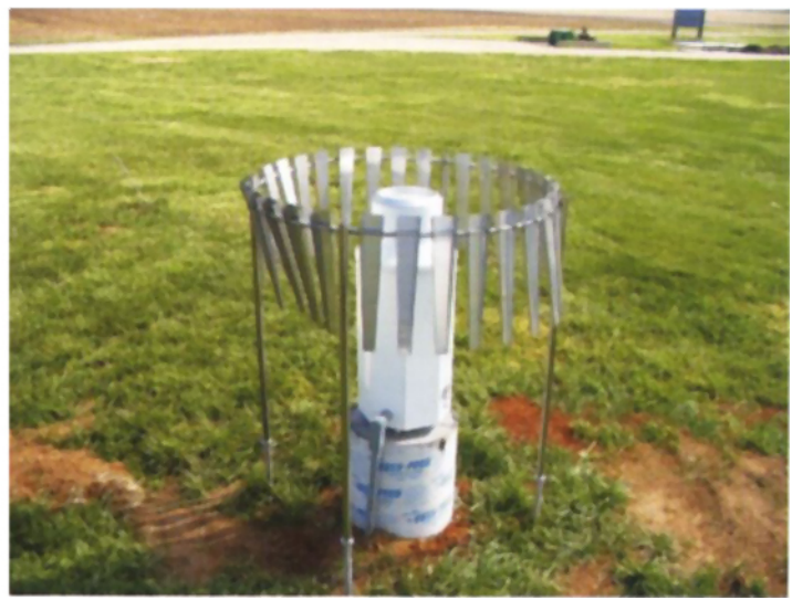
Weighing bucket rain gauge with alter shield.
