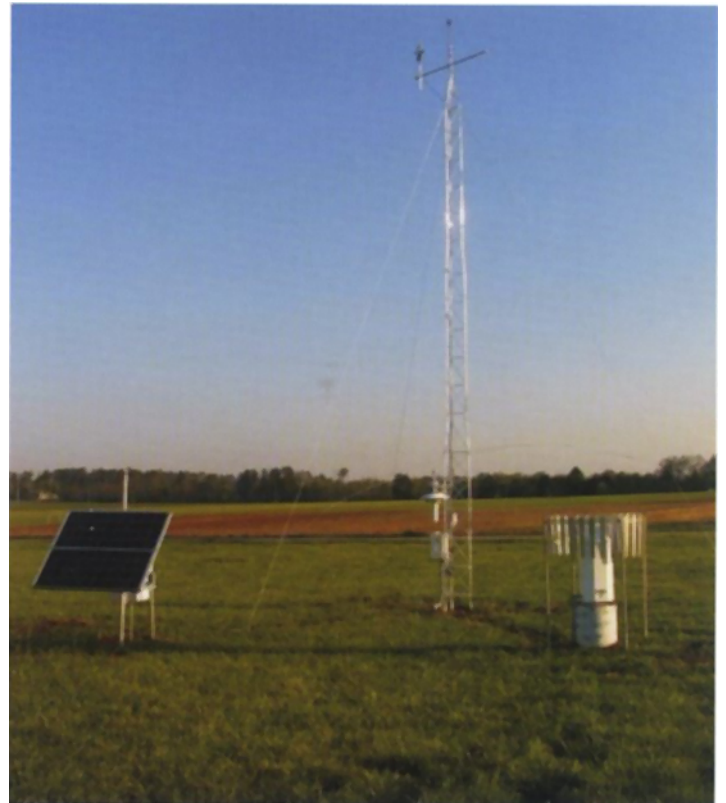
Completed Mesonet test station showing the tower with instruments, weighing bucket rain gauge with single alter wind shields, and solar panels. Wind shields allow for the reduction of winds on rainfall measurement known as undercatch. Typically, wind causes lower rainfall measurements.
