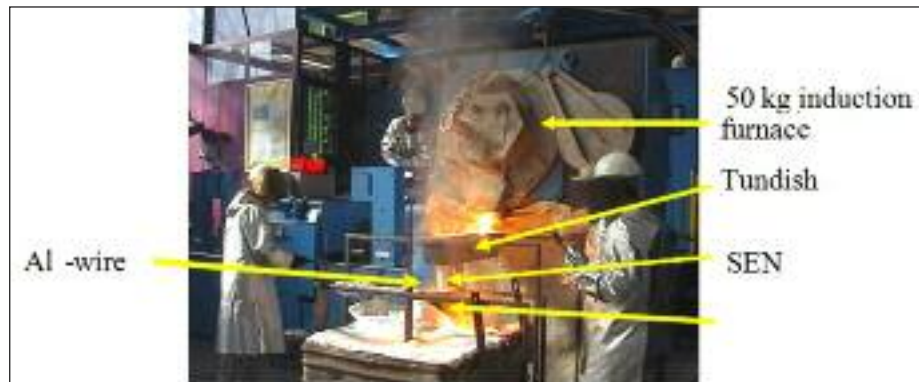
FIG. 4 Laboratory trial at 0.5 t induction furnace at IEHK of RWTH Aachen University.
