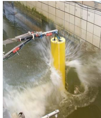
Figure 1: Physical modeling (1:12) of the tripod structure in the large wave flume (left) and in the CFD model (right).
