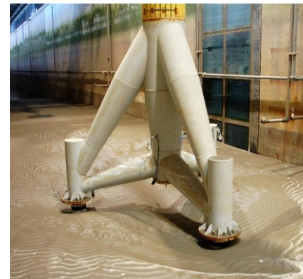
Figure 1: Tripod model structure and scour pattern in the GWK wave flume
