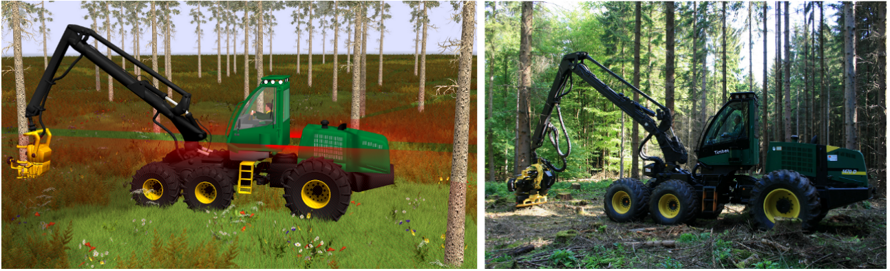
Figure 2. Virtual and real testbeds; left: Simulated forest machine with laser scanner visualization; right: photo of the real harvester with mounted laser scanners.
