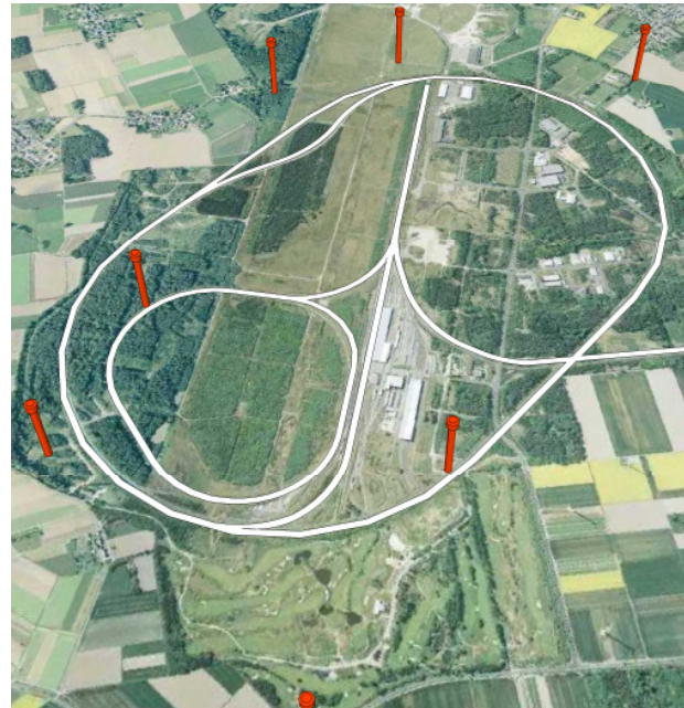
Figure 2: Illustration of the railGATEs pseudolites, © RWTH/IRT
