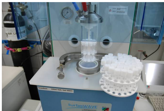
Fig. 3: The turboWAVE system and a 40 position ultraCLAVE rack for comparison reasons
