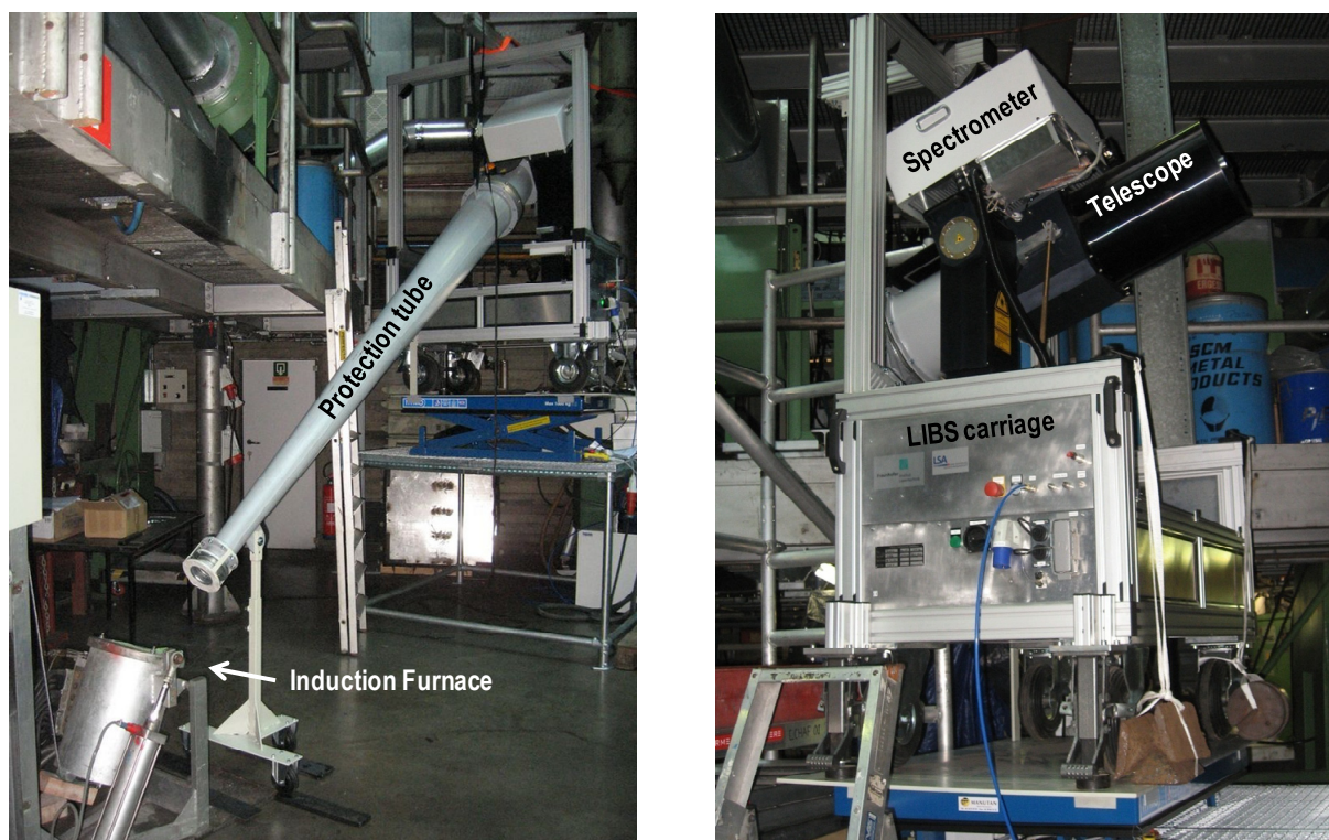
Figure 3: View of the pilot set-up for LIBS measurements on liquid hot metal
