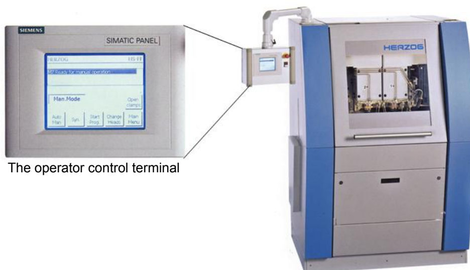
The Herzog HS-FF2000 milling machine
