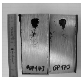
Porosity/shrinkage in the upper part of a LUS
