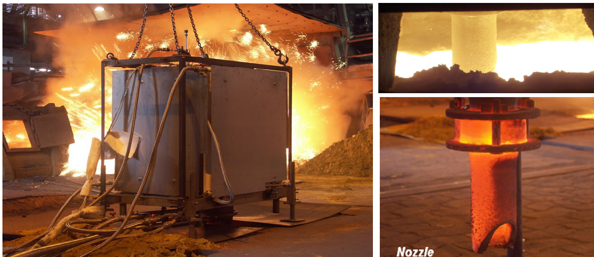
Figure 6: View of the LIBS measuring device on top of the ArcelorMittal Gent blast furnace runner - to the right, views of the nozzle during and after the test.
