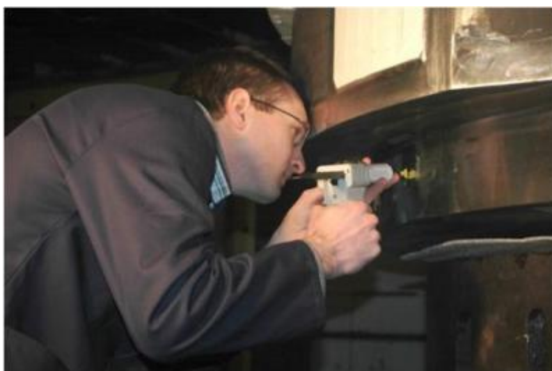
Figure 17 Taking of replicas
