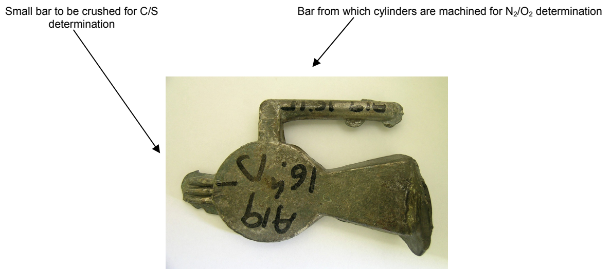
Figure 6 – Cast iron test piece with lateral cylindrical device
