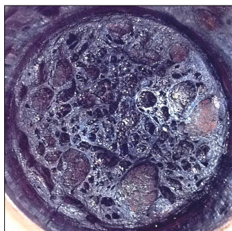
Fig.1 – Oxidized stainless steel in the crucible
