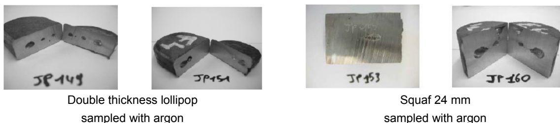
Figure 7: Location of the macro-porosity in the double thickness lollipop (left) and squaf 24 mm sample (right) taken with IDCAS.
