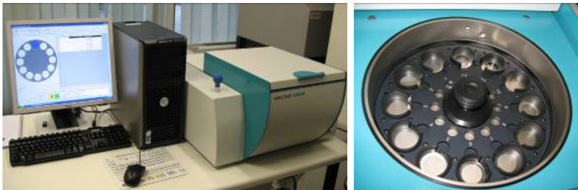
Picture 1: illustration of XRF system used at OCAS
