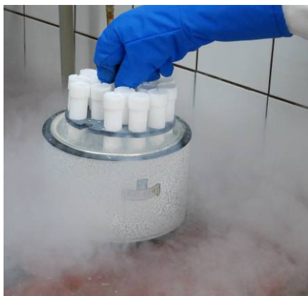
Fig. 5: Preparation of FeB for the ultraCLAVE
