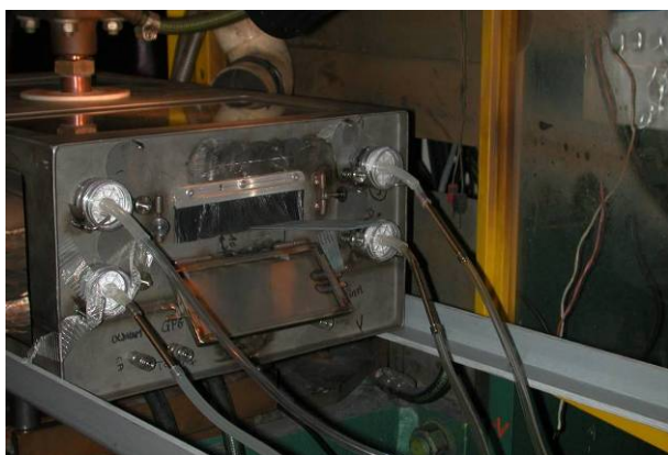
Figure 2: Sampling box of 60 litres made of glass and stainless steel
