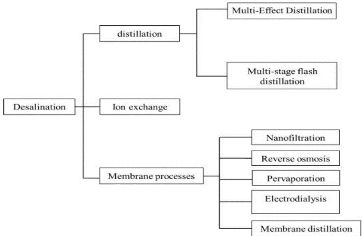
Figure 2.1: Classification of water desalination technology process [2].
