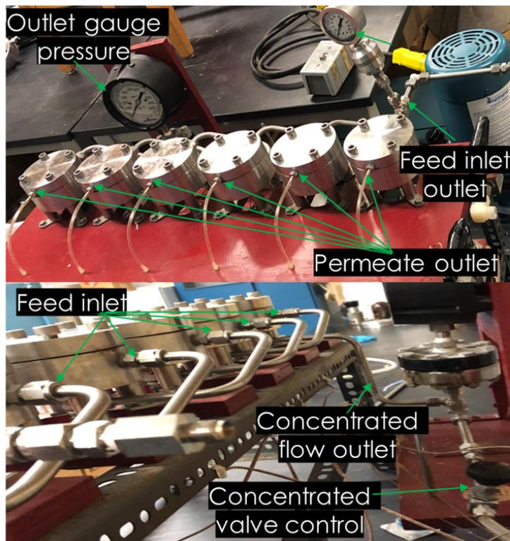
Figure 3.2: Front and back view of experimental set-up.
