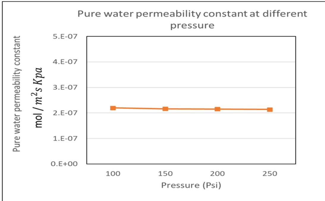
Figure 4.3: Pure water permeability coefficient of RO membranes at feed water flow rate 1.35 ml/sec.
