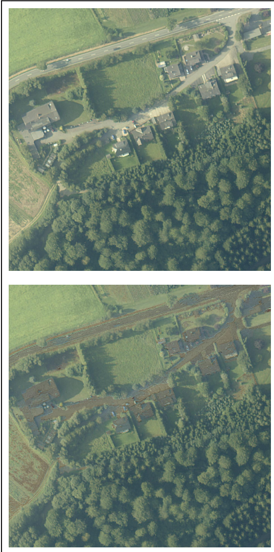
Figure 3. RGB True-Ortho-Photo and Image after Colour-Tone-Based Brightness Reduction
