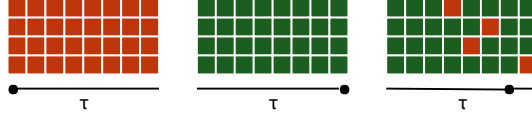
Figure P4.6: Example of how an anomaly detection visualization changes with different threshold settings; the rightmost setting corresponds to how a user would likely set the slider manually
