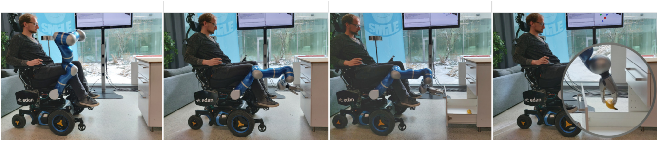
Fig. 8. Picture series of the task open drawer . The task is automatically activated, as soon as the user moves the end-effector close to the drawers handle. Once the handle is reached, motion is limited to opening the drawer. Afterwards, the object is picked from the drawer using manual control.
