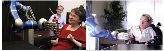
Fig. 4. The DLR LWR-III as an assistive device. Left: Footage from the Braingate2 Clinical Trial [14]. Right: Footage from our study on sEMG-based interfaces for people with severe muscular atrophy [17].
