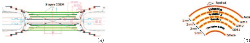
Fig. 1. – Scheme of the three CGEM layers positions (a), and construction detail of each CGEM layer (b).
