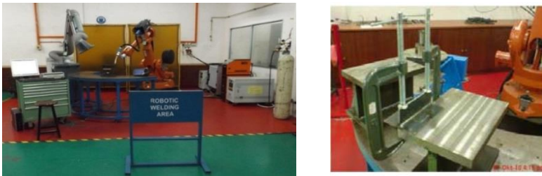
Figure 7 : Robotic welding apparatus: ABB IRB 2400/16, KEMMPI ProMIG 540 MXE and shielding gas (80 % Ar and 20 % CO 2 )
