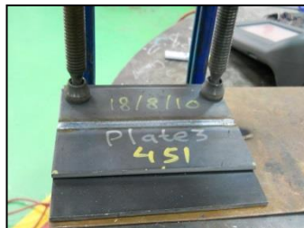
Figure 2: Clamping conditions applied for butt joint
