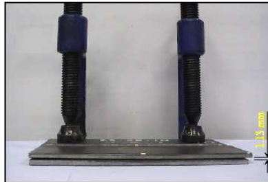
Figure 9: Angular distortion of specimen
