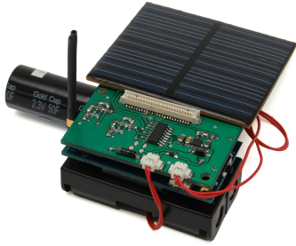
Fig. 1. Energy Harvesting Platform for the IRIS node
