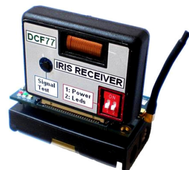
Figure 1. DCF77 receiver hardware developed for IRIS nodes
