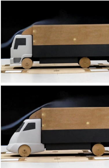
Figure 26. Visualisation of aerodynamics in the wind tunnel for a box truck with spoiler. [6]
