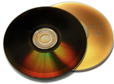
(d) Picture of a DVD-RAM (picture taken by Dominic Lencer). The reflectivity contrast between the written (inner) and unwritten (crystalline) regions is obvious.
