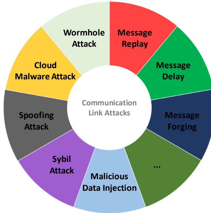
Figure 2.4: Different types of attacks toward the communication link for transmitting timestamps for clock synchronization.
