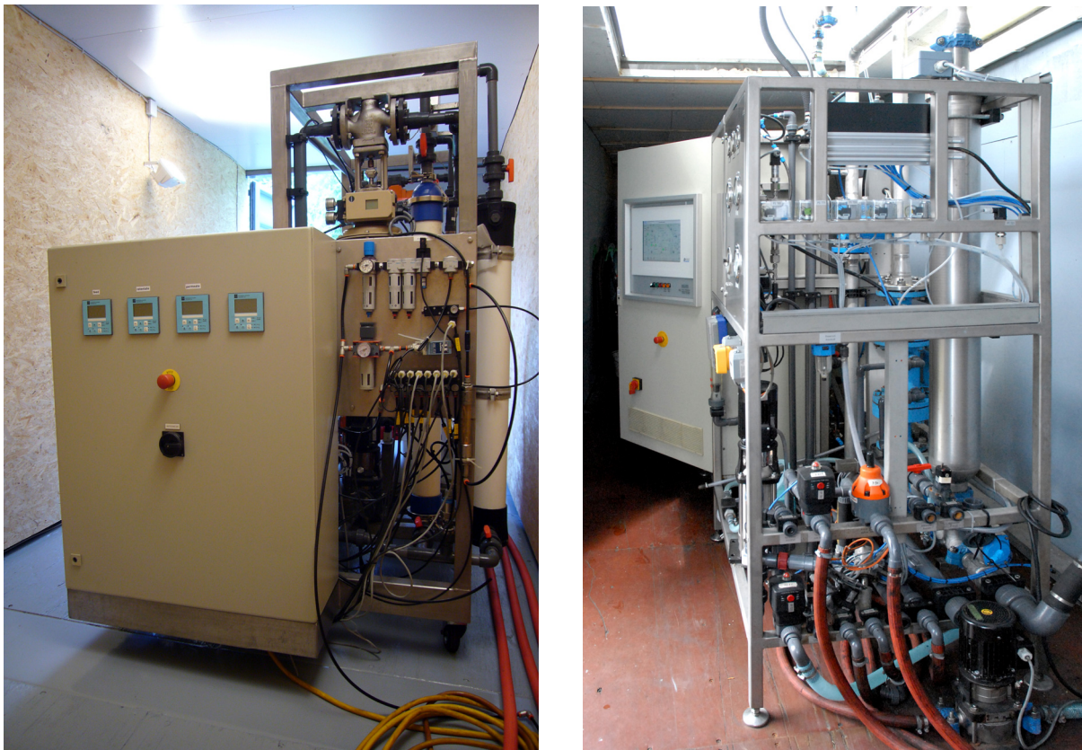
Fig 7.1 Fully automated 4" pilot plant (left) and 8" pilot plant (right) for capillary NF tests at WWTP Aachen Soers
