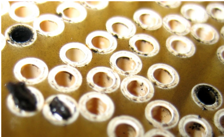
Fig 7.12 PAC/NF: Partial blocking of capillaries on the influent side of the NF module (After approx. 3000 operating hours, condition after backflushing)
