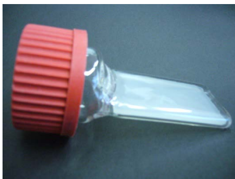
Figure 2-2: Picture of chamber for loading siloxane-plates with organic compounds.
