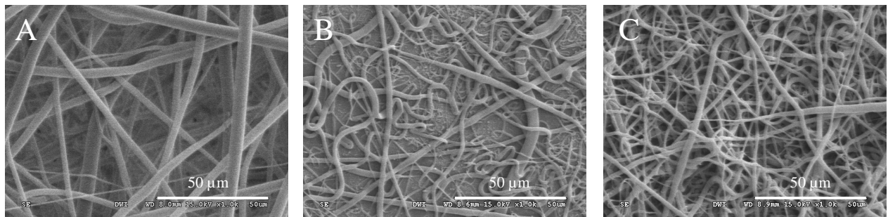
Figure 5-13: SEM graphs for polypropylene electrospun fibers containing different types of nucleating agents electrospun at electric field strength of 3.75\text{ kV}/\text{cm} at the applied voltage of 30\text{ kV} and the distance between electrodes was 8\text{ cm} . A: HL 504 FB + 0.2 wt.-% Irgastab NA 11 (Fiber diameter: 2.98 \pm 1.54\text{ }\mu\text{m} ), B: HL 504 FB + 0.2 wt.-% HPN-68L (Fiber diameter: 0.98 \pm 0.51\text{ }\mu\text{m} ) and C: HL 504 FB + 0.2 wt.-% Irgaclear DM (Fiber diameter: 1.52 \pm 0.70\text{ }\mu\text{m} ).
