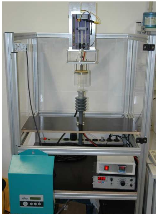
Figure 1: Electrospinning machine designed by ITA (Source: ITA, RWTH-Aachen, Dipl. Ing. Christoph Hacker, Dipl. Ing. Philip Jungbecker and Prof. Dr. Ing. Thomas Gries)
