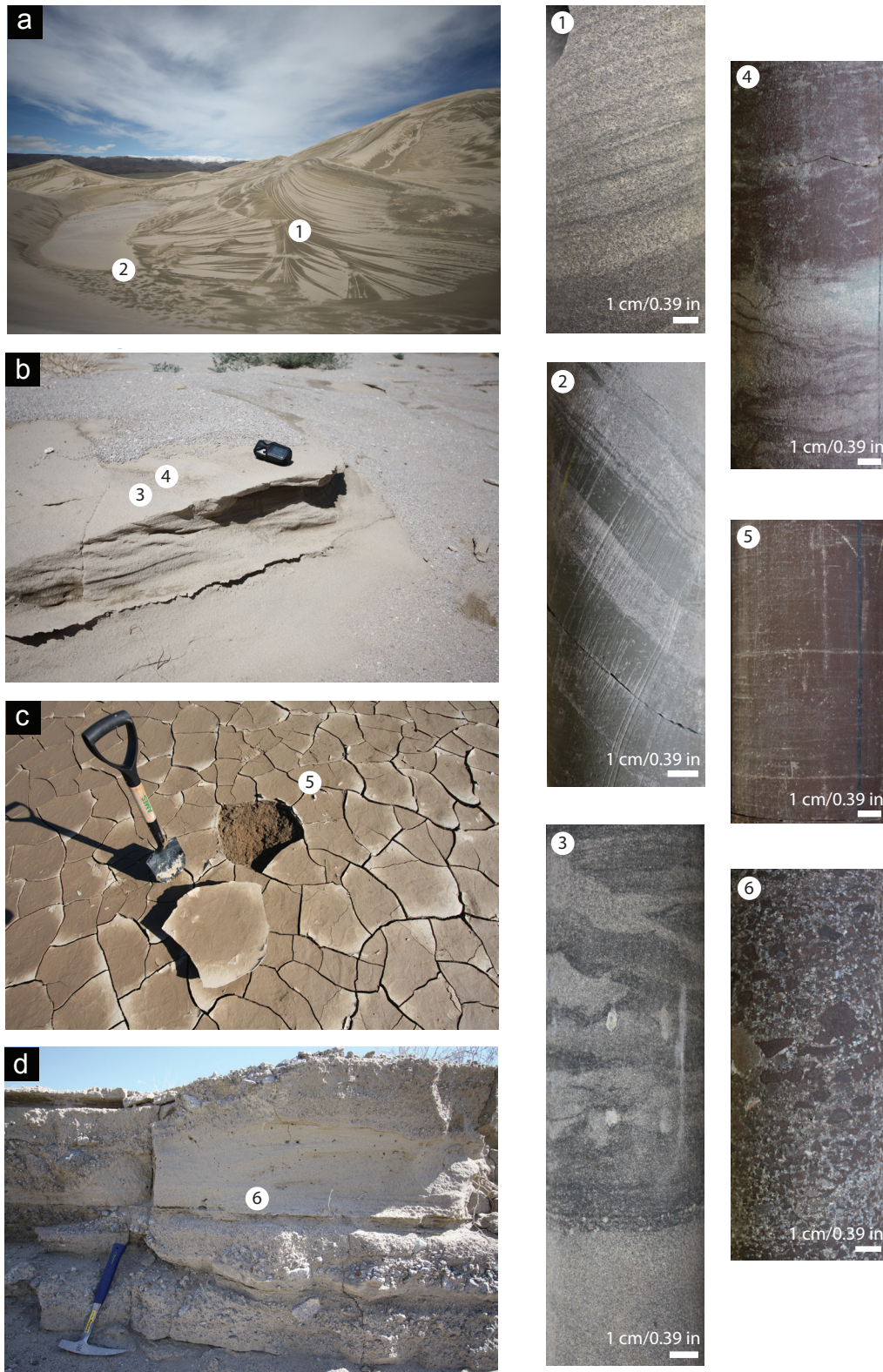
Fig. 4.5: Comparison of sedimentary facies of the Panamint Valley and the study area in Germany. Photo locations a-d marked in Fig. 4.3. Core photos of the Wells C1 and C2: (1) dune deposits, (2) pond margin deposits with dune deposits migrating into the pond. Note the deviation. (3) damp sandflat. (4) wet sandflat, (5) mudflat, (6) low energy fluvial deposits.
