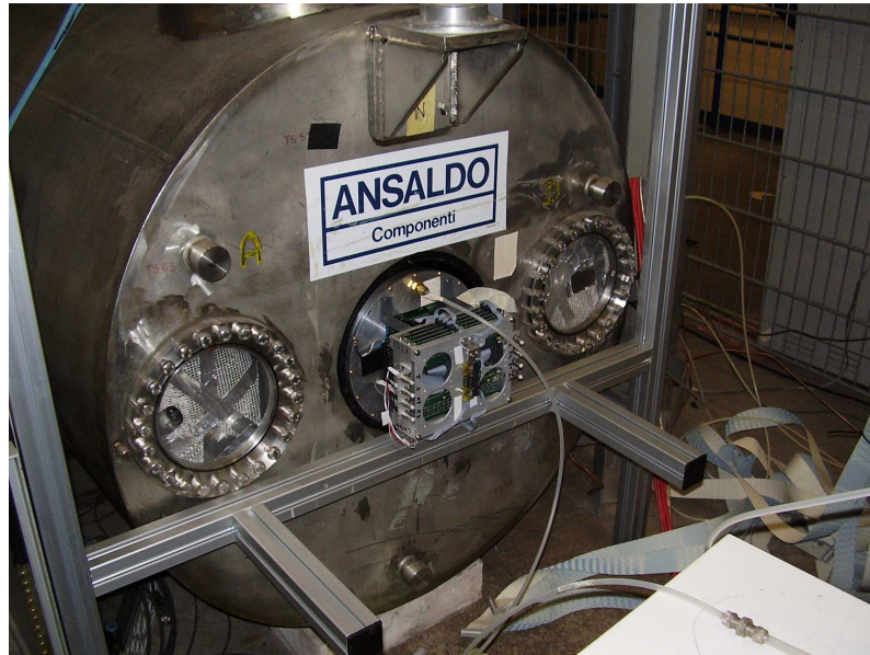
Figure 4.11: The TPC in the bore of the 5 T superconducting magnet at DESY Hamburg.
