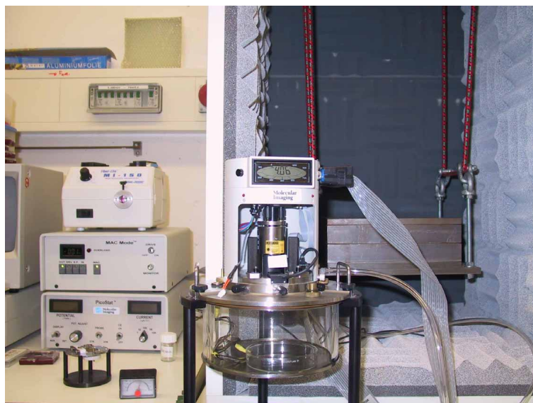
Figure 6.1: Experimental setup: Molecular Imaging PicoSPM with environmental chamber. The Petri-dish inside the chamber is used to deliver the solvent vapors. In the background is the vibration damping system based on bungee cords, mounted into a soundproof box
