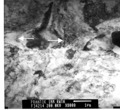
Fig. 21 Localized process of dislocation rearrangements and nucleation.
