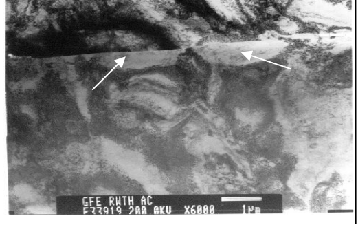
Fig. 22 b) possible grain boundary nucleation along a grain boundary
