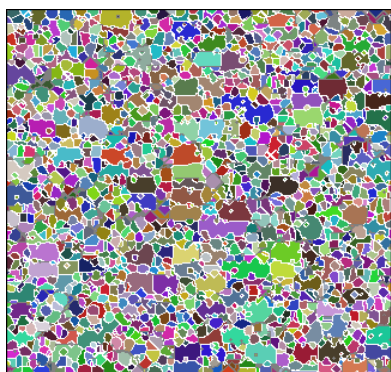
Fig. 50 a) The effect of nuclei orientation and initial grain size on simulated recrystallization microstructure. 60-micrometer initial grain size. Nuclei orientation randomly selected.
