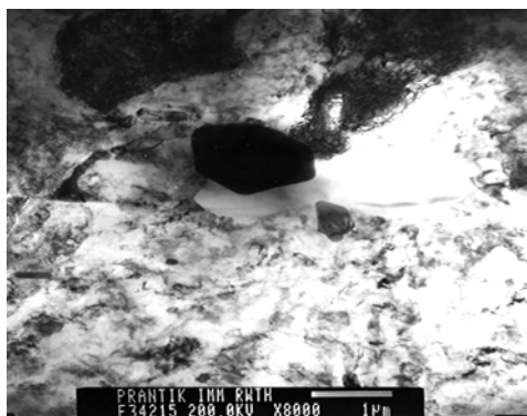
Fig. 25 a) The nucleation of grain near precipitate.
