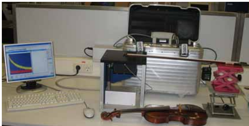
Fig. 5.7 The NMR-MOUSE setup to measure the depth profiles for the violins and bows. It consists of the NMR-MOUSE which is placed on top of a movable plate, which, controlled by a step motor, can automatically move the sensor with respect to the sample so that depth profiles can be acquired.
