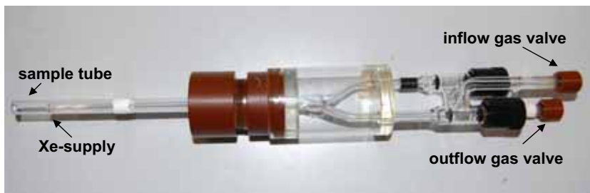
Fig. 4.2 Probe for the hyperpolarized ^{129}\text{Xe} NMR measurements. The Xe flow is achieved with the help of an inflow gas tube and an outflow gas tube.
