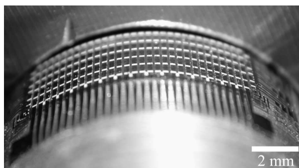
Figure 6.5: Bending of a complete system consisting of a silicon chip with a thickness of approximately 20\ \mu\text{m} , soldered to a polyimide tape. The image shows mechanical bending with a radius of 7.5 mm.
