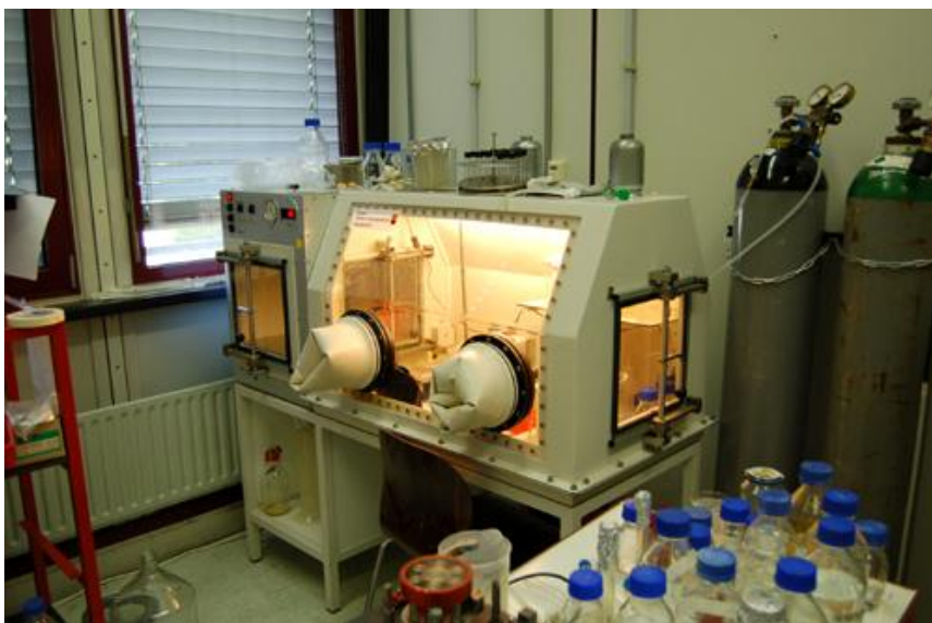
Figure 3.12: The house-built anaerobic bench, where all the handling and preparation steps of the biomass containing the enoate reductase enzymes were carried.
