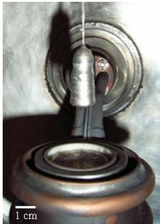
Figure 2.13: \beta -Al-Mg single crystal grown by means of the Czochralski technique. The inductive heater containing crucible and residual melt is also visible.
