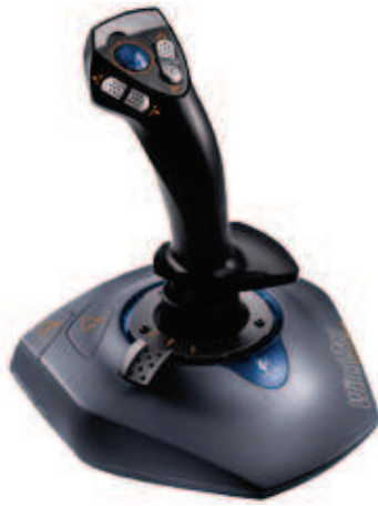
Fig. 4. An analog joystick measures absolute tilt of the stick in the rX , rY dimensions.
