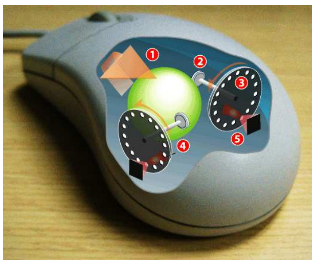
Fig. 3. An optical-mechanical mouse: (1) Motion across the desktop surface moves the ball. (2) Grips transfer the ball movement to turn (3) optical encoding disks. (4) Infrared LEDs shine through the holes. (5) Infrared sensors accumulates light pulses and converts them into X, Y motion. (Source: Wikipedia)
