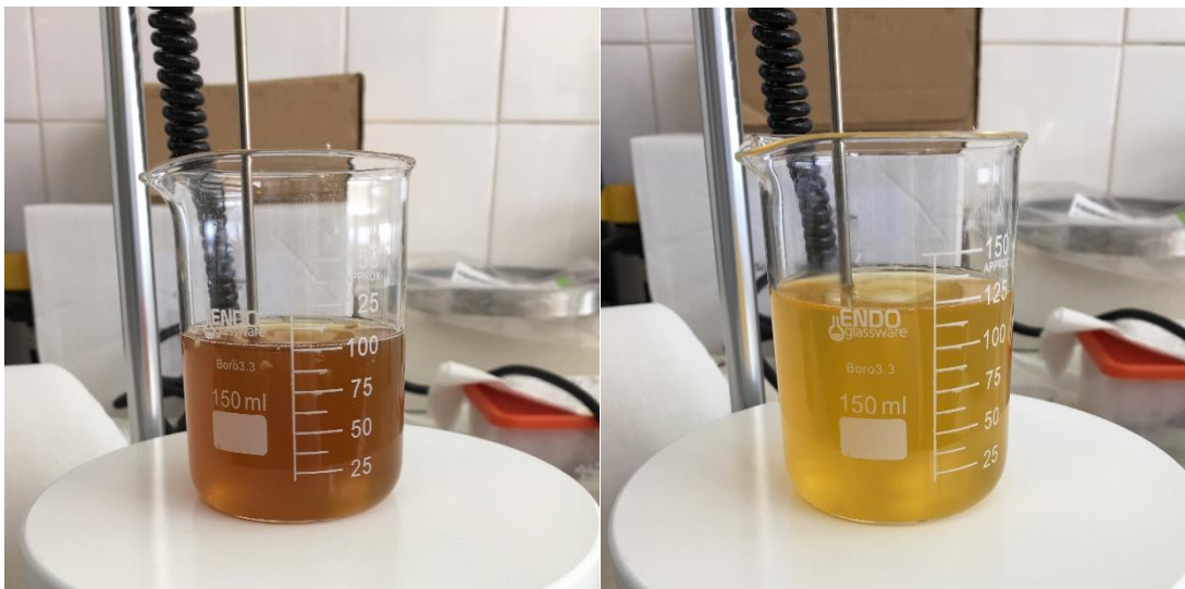
Figure 3.12: Solution of arabinoxylan before the addition of hydrogen peroxide (left) and after the reaction time of 2h at 45°C (right).
