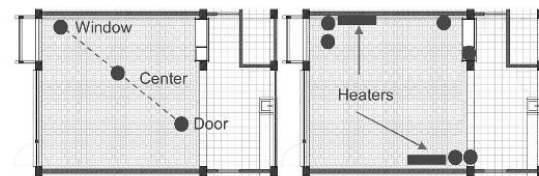
Fig. 7. (left) Hygrothermal monitoring sensors; (right) Energy consumption sensors and heaters.
