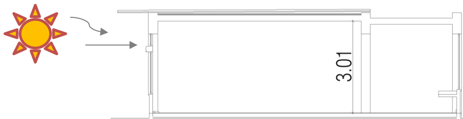
Figure 46 – Inlet air below the roof overhang.
