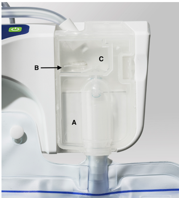
FIGURE 8. The measuring chamber (A, lower 2/3) of the automatic urinometer (Sippi ® , Observe Medical, Gothenburg, Sweden) with a water-soluble capsule (B) containing medium viscosity silicone oil in its antechamber (C) upper 1/3). (Reprinted with permission from Observe Medical).
