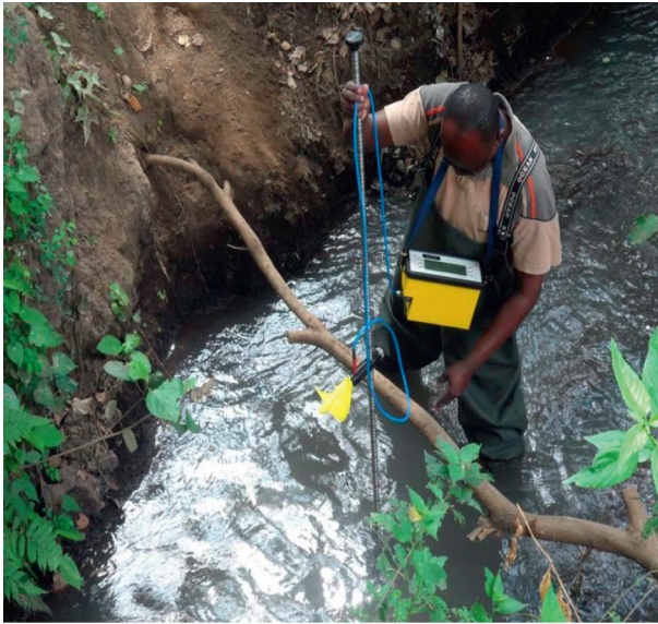
FIGURE 3: Water flow measurement at traditional canal using current meter.
