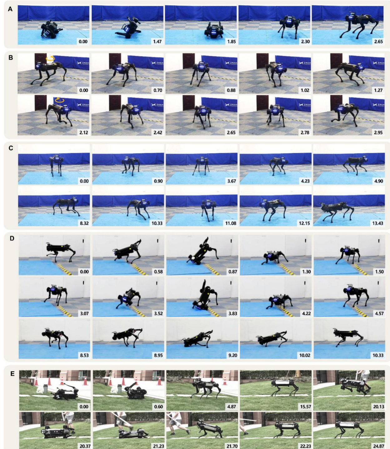
Fig. 5. Dynamically synthesised MELA policy running on a real quadruped robot and demonstrating adaptive and agile locomotion behaviours. (A) Successful fall recovery performed by the MELA expert,
