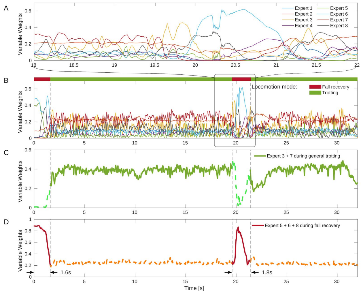
Fig. S13. Continuous and variable weights of all experts during the real MELA experiment on grass (Fig. 5E). (A) The variable activations within a zoomed period to show the transition of weights between multiple experts. (B) The variable activations of the entire multimodal locomotion with trotting and fall recovery during a target-following task. (C-D) The activation levels of paired weights from collaborating experts, where the expert groups (3, 7) and (5, 6, 8) cooperated together in trotting and fall recovery, respectively.
