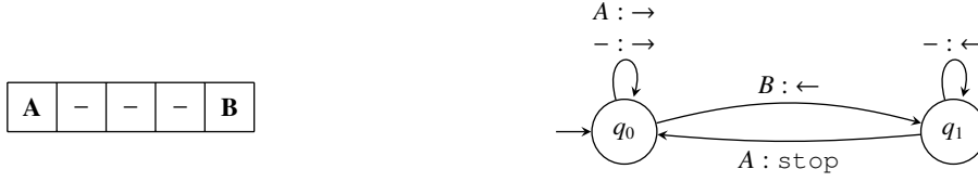
Figure 1: Left : A planning problem where the agent is initially in cell A, and the goal is to visit cell B and go back to cell A. At each state, possible observations are A, B, or -. Right : A correct finite state controller for this problem. The circles are controller states, and an edge q \xrightarrow{o} q' means “do a when the observation is o in controller state q , and then switch to controller state q' .” The reader may observe that this controller works for any number of states between A and B in the domain, e.g., for (A, -, B) as well as (A, -, -, -, B) .
