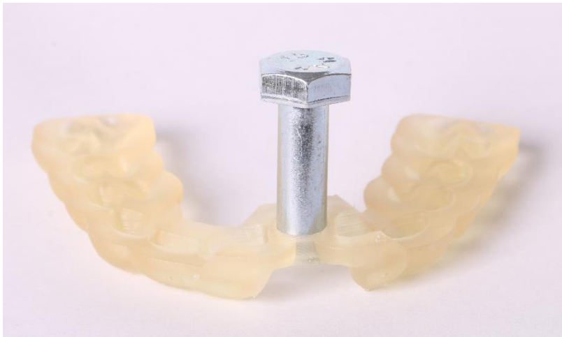
Figure 2. 3D printed surgical guide with stainless-steel bolt secured in the guide tube.
