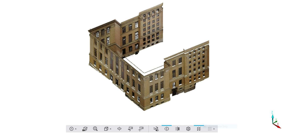
Figure 3.8 – Isometric view of Cushing Memorial Library trimmed point cloud looking north, created using the FARO3D Focus x330 HDR.
