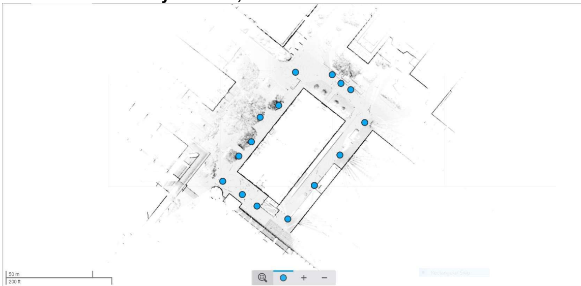
Figure 3.6 – FARO Scene Overview Map showing the scan locations used on Animal Husbandry Pavilion, the FARO Focus 3D data set is shown.
