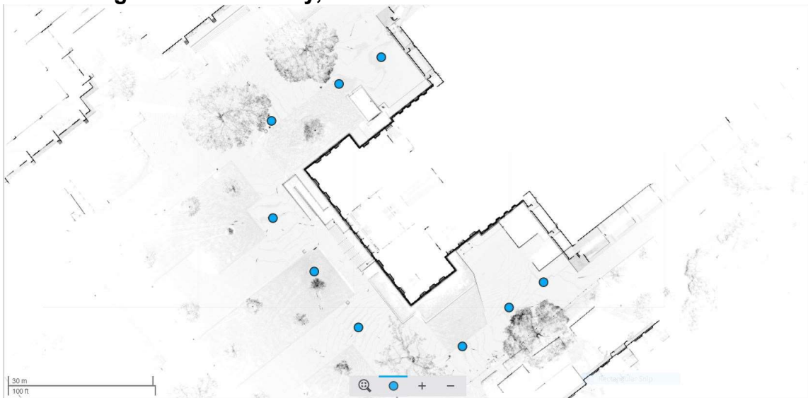
Figure 3.4 – FARO Scene Overview Map showing the scan locations used on Cushing Memorial Library, the FARO Focus 3D data set is shown.
