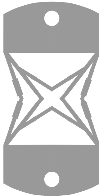
Figure 6.7: Example of a SPIDRS-generated structural module which features varying member thicknesses determined by the algorithm in a manner consistent with material assignments.
